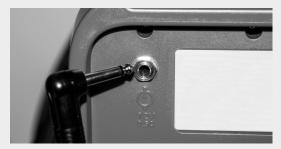
• Plug the connector into the (12V. 0,5A) jack.
