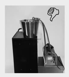
The machine must be on a higher level than the water tank.
