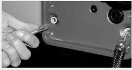
• Press the cooling adapters into the sockets on the back of the machine, then pull on the hoses to check that they are firmly attached.
