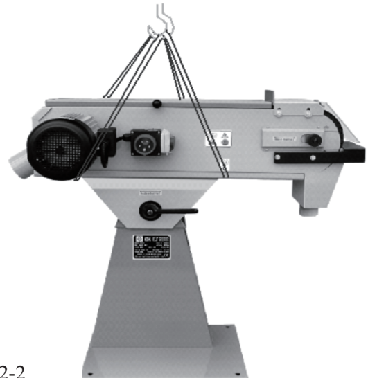
Fig. 2-2 Transportation sketch with a crane (After unpacking)
