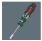
High-quality bit-holding screwdriver with a strong permanent magnet that holds bits securely. Multi-component Kraftform handle for comfortable, ergonomic work. Suitable for bits with 1/4" external hexagon drive as per DIN ISO 1173-C 6.3. Up to six bits can be stored in the magazine integrated in the handle.
