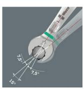
Thanks the pivoted to 7.5° the double mouths, hexagon improved geometry and an application method (placement screwdriving - rotation - replacement - screwdriving - rotation etc), even screwdriving situations that have a pivoting angle of less than 30° can be solved.
