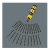
The robust bit mounting is suitable for bits with 1/4" external hexagon drive as per DIN ISO 1173-C 6.3 and E 6.3. The interchangeable blade system means low weight, reduced space requirement and high flexibility for the user.
