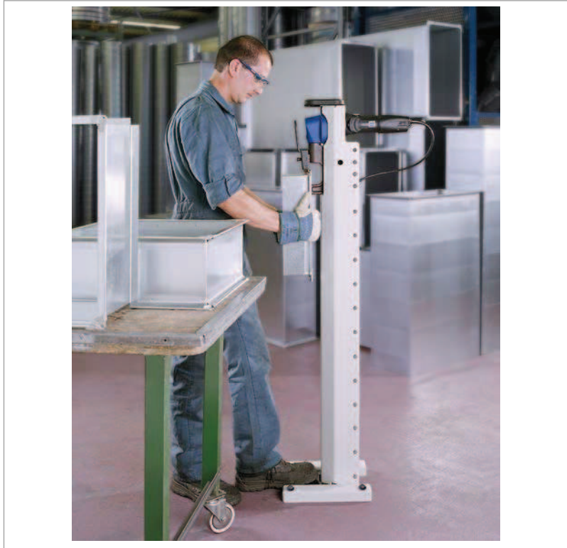
TruTool TF 350 with joining station
