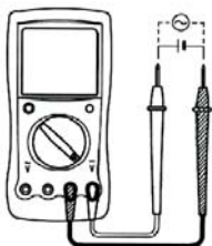
Fig 1. Voltage measurement DC and AC
